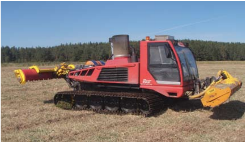
Figure 3. New machinery of Lännen Järviperkaus that can crush and harrow coastline reed beds. The machinery was used in important areas for Dunlin Calidris alpina in Mietoistenlahti Bay in 2010. Photo: Iiro Ikonen.
