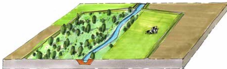
Figure 1. Lowered floodplain (agricultural or natural) for water retention (drawing: Dirk Oomen, Stroming BV).
