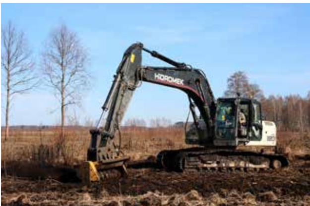
Figure 16 and 17. Stump mulching equipment at work (13.03.2014). Photo: I. Priedniece, E. Račinskis
